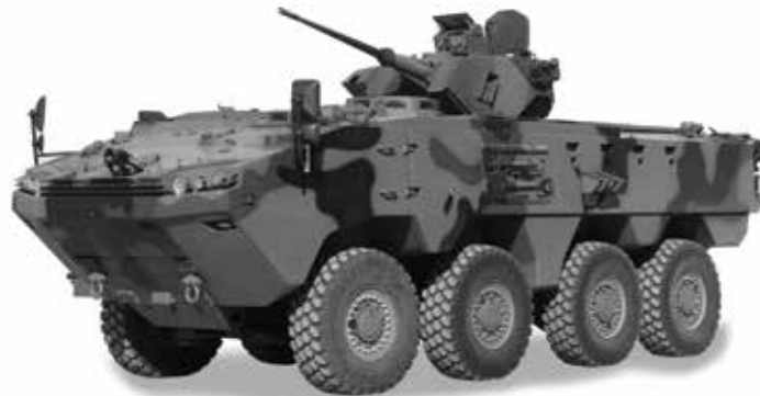
Otokar Arma 8x8 armoured combat vehicle
