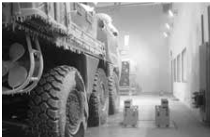
Climate controlled Test Chamber with Dynamometer
