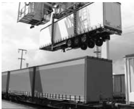
Otokar semi-trailer suitable for railway transportation
